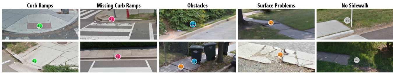
Figure 3. Project Sidewalk has five primary color-coded label types: curb ramps , missing curb ramps , obstacles , surface problems , and no sidewalk . The images above are example accessibility issues found by users in our public deployment.
